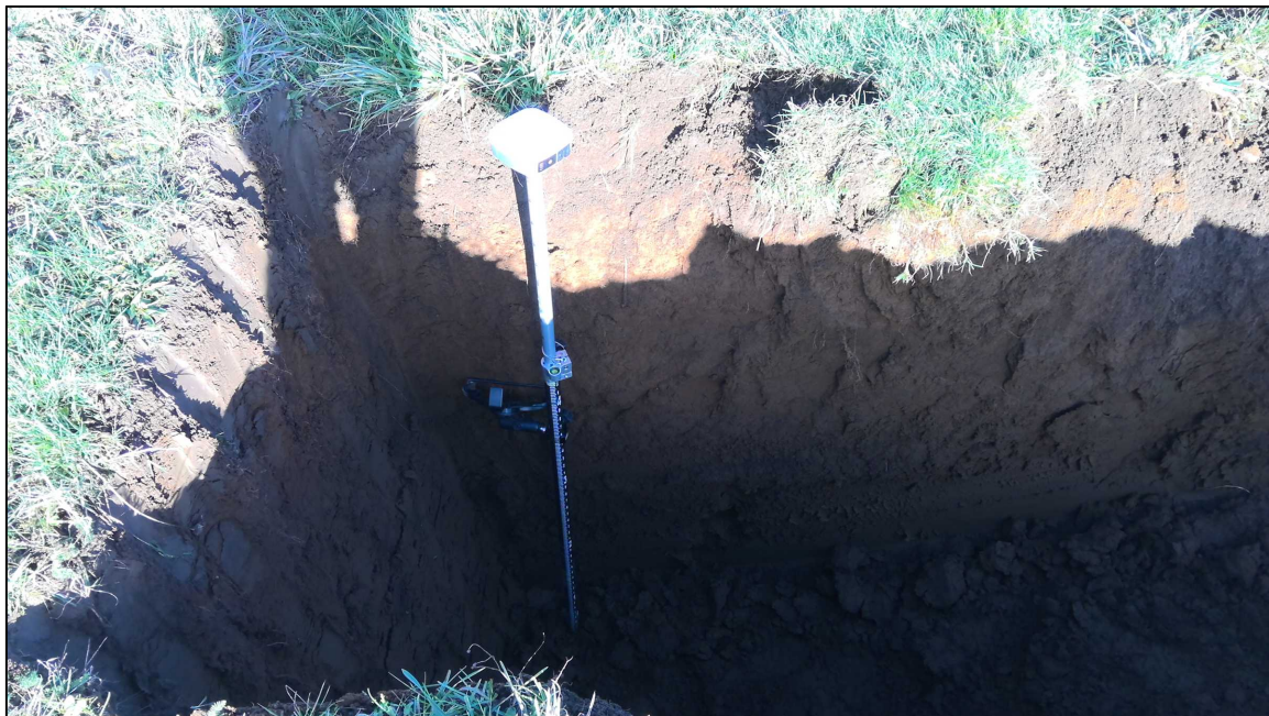
FIGURE 12--SOIL TEST PIT IN PROPOSED DRAINFIELD AREA. SOILS DETERMINED TO BE CONSISTENT WITH CHEHALIS-MAYTOWN COMPLEX AND FOUND TO BE WELL DRAINED SILT LOAM TO LOAM AT A DEPTH GREATER THAN 72 INCHES. PHOTO DATED 1-15-26
