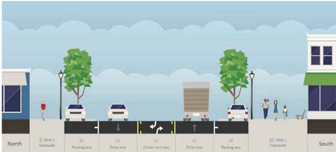
Figure 2: Highway 12 Cross-Section Concept, Rochester, WA (Source: Thurston Regional Planning Council)
